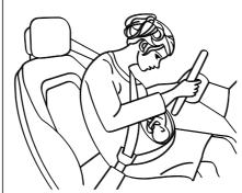
Pregnant women should follow special instructions from their doctors when driving or riding in vehicles. Three-point seat belts should be used when driving or riding in a vehicle. The shoulder seat belts should be placed in the appropriate place of the chest and the seat belts in the pelvis should be as low as possible. Seat belts must be flat and sit straight back to reduce the risk of injury to the mother and fetus from a crash or inflatable airbags.
