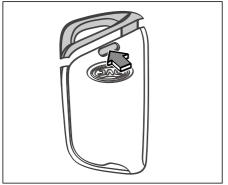
2. Twist the upper shell clasp of the shell gently, and then open the shell at the gap of the shell.
