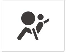
The airbag warning light monitors the status of the airbag system, the circuit of the belt pre-tightening system and all related circuits.
