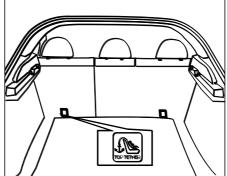
The top strap is connected to a retaining ring on the back of the back seat by a retaining hook.
