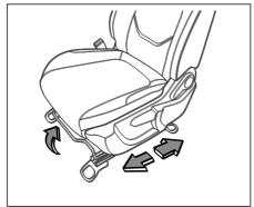
Lift up the pull rod in front of the seat and move seat back and forth. Seat should be fixed after pull rod is released.
