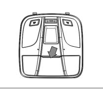
The glasses box is located on the roof console. Press the top of the lid to open the glasses box.
