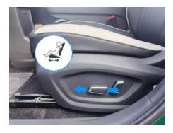
Push the switch in the arrow-indicated direction to move the seat back and forth.
