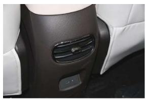
The USB port can only be used for charging and not for connection to the multimedia system.
