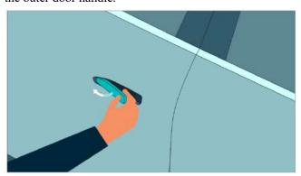
The outer door handle will automatically retract after the vehicle is locked, the speed exceeds 4km/h or it has been retracted for more than 30s.
