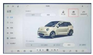
When this function is activated, the window glass can only be raised and lowered through the driver's side window control main switch, and the passenger's side window regulator switch will not work.
