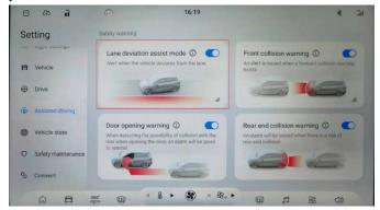
The mode of lane departure warning can be set as "warning", "deviation correction" or "warning + deviation correction" in the lower right corner of this function interface according to requirements, and the sensitivity of lane departure warning can be set as "low" or "high".
