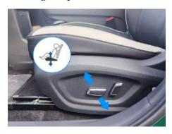
Press the switch along the direction indicated by the arrow, and the overall height of the seat will rise up or go down.
