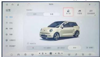
When the vehicle is in unlocked state and all doors are closed, press the switch on the central control panel to lock the vehicle. In case of door locking, the switch icon will become locked  $\Theta$ .
