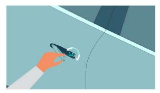
4. When locking, press the front area of the outer door handle and turn the mechanical key counterclockwise to lock the driver side door.
