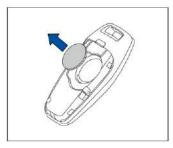
3. Press one side of the battery with finger or screwdriver to remove it.
