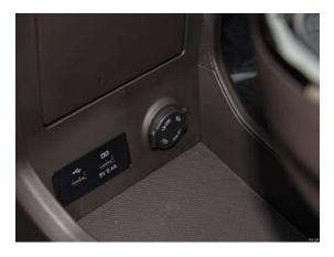
The USB port supports data transmission with MP5.
