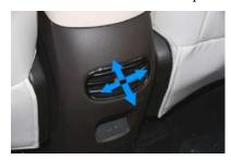
The air outlet angle can be adjusted by moving the adjusting sheet in the center of the air outlet left and right. Slide the toggle button of the air outlet to the left or right limit position to close the air outlet.
